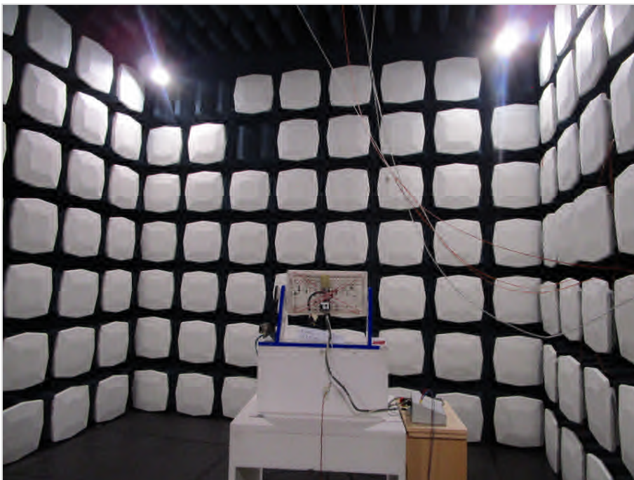
Photograph 4: EUT test setup in the fully anechoic chamber, overview
