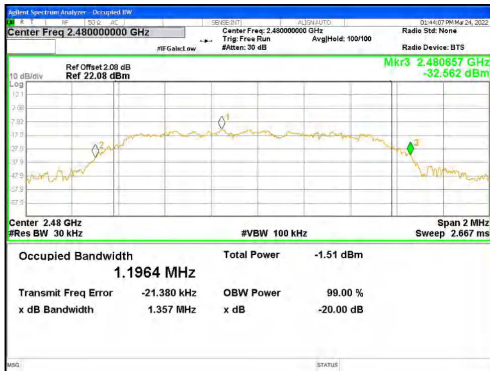
-20dB Bandwidth NVNT 3-DH1 2402MHz Ant1
