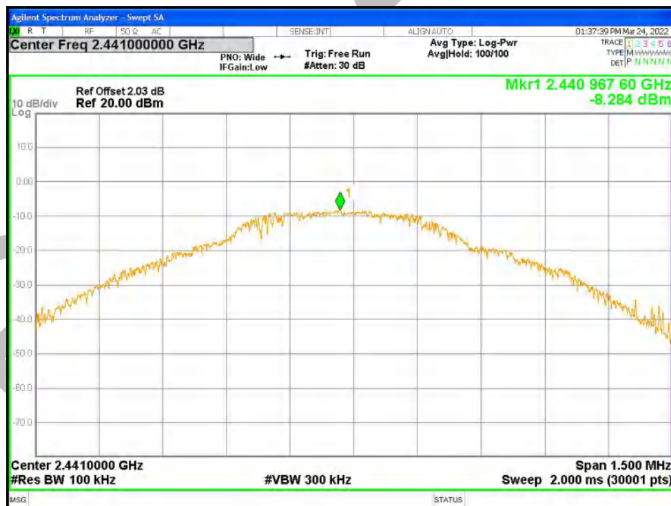
Tx. Spurious NVNT 1-DH1 2441MHz Ant1 Emission
