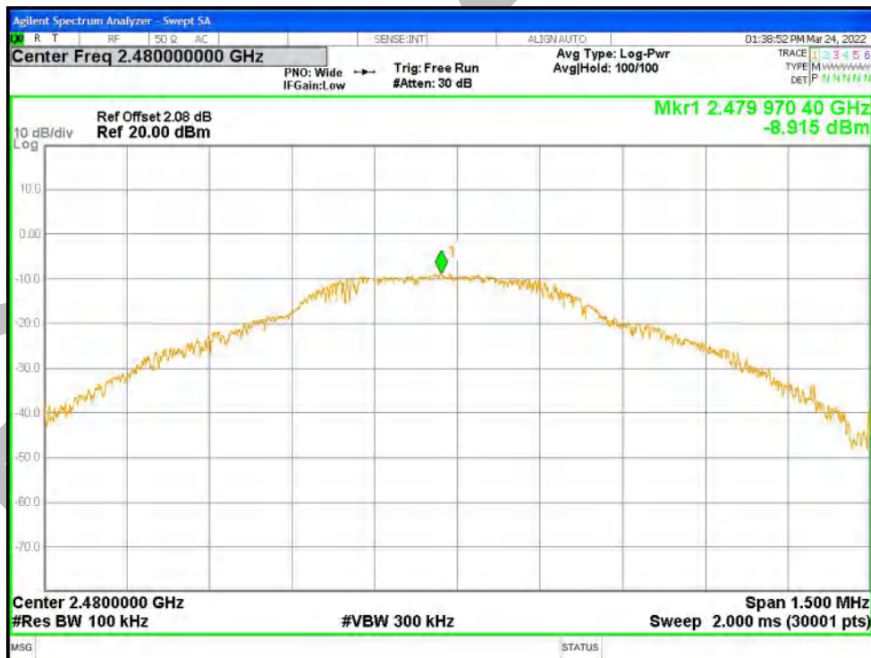
Tx. Spurious NVNT 1-DH1 2480MHz Ant1 Emission
