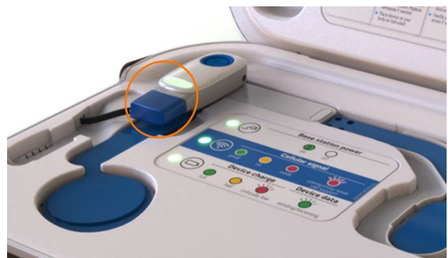
Figure 22 a-c. a-b) Plugging the Base Station into the wall and c) Magnetic charging and LED indications in the Base Station.
