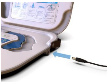
Figure 22 a-c. a-b) Plugging the Base Station into the wall and c) Magnetic charging and LED indications in the Base Station.
