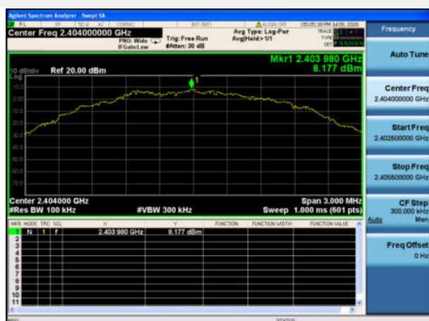
GFSK (BLE 2Mbps) LOW CHANNEL, CARRIER LEVEL
