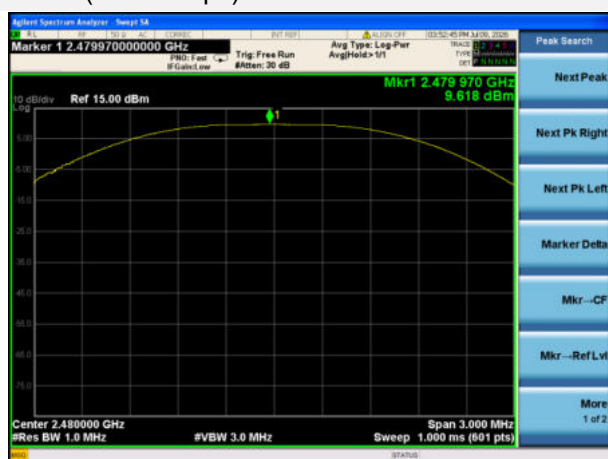
GFSK (BLE 1Mbps) HIGH CHANNEL
