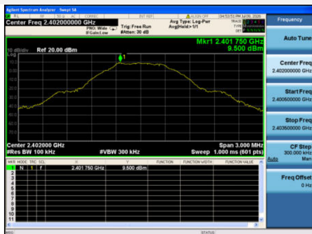
GFSK (BLE 1Mbps) LOW CHANNEL, CARRIER LEVEL
