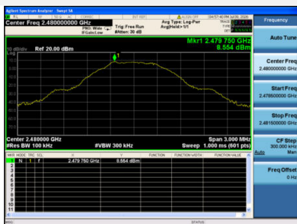
GFSK (BLE 1Mbps) HIGH CHANNEL, CARRIER LEVEL
