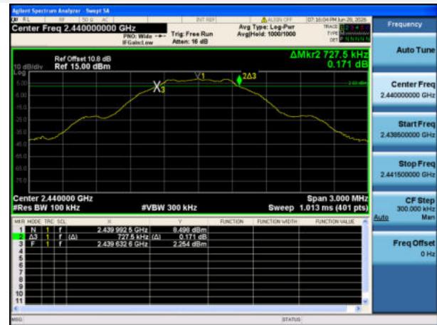
GFSK (BLE 1Mbps) MIDDLE CHANNEL
