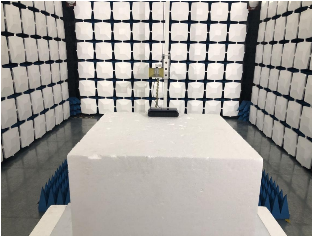
Above 1GHz for radiated emission test setup
