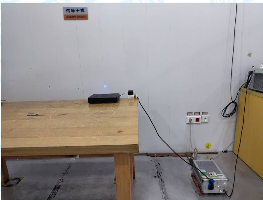
Photo of Setup for Conducted Emission
