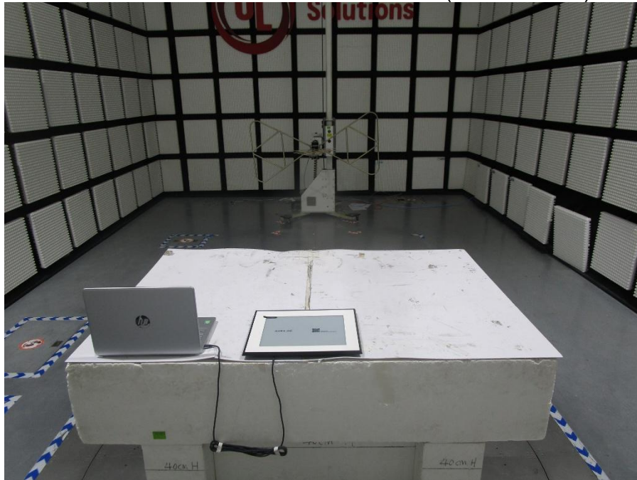
RADIATED RF MEASUREMENT SETUP (Below 30MHz)
