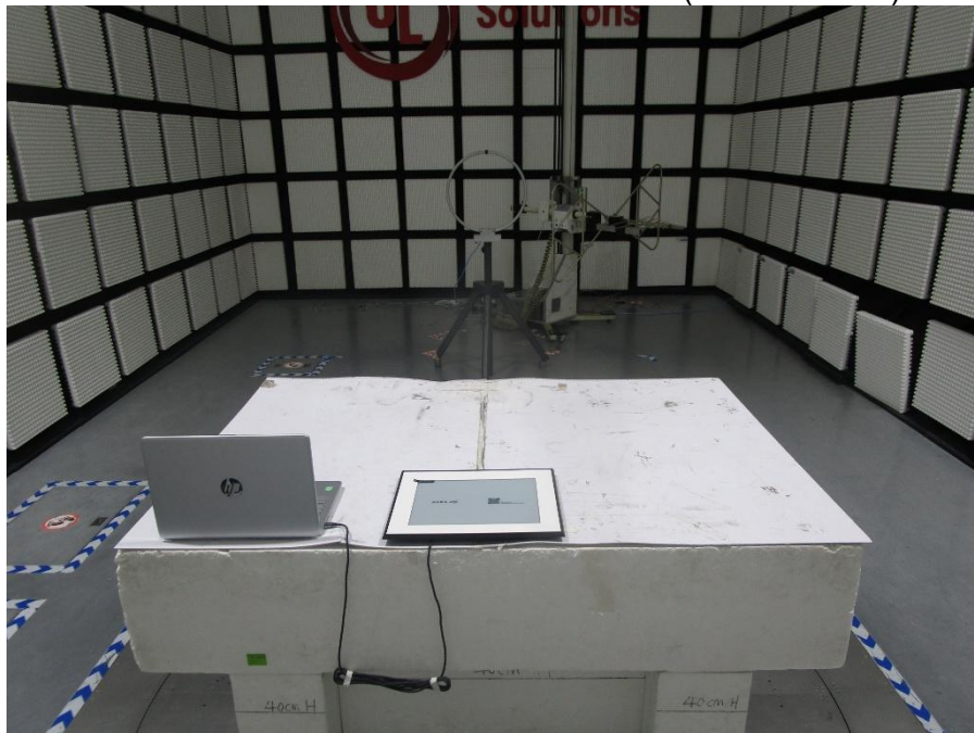
RADIATED RF MEASUREMENT SETUP (Below 30MHz)
