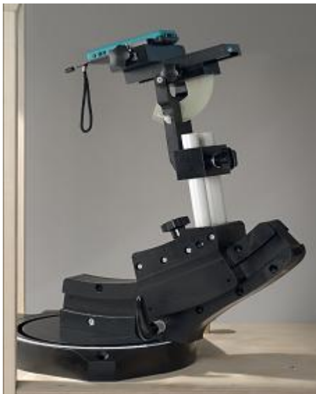
F-2. Device Holder for Transmitters
