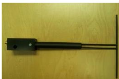
Figure 1 – MVG COMOSAR Validation Dipole
