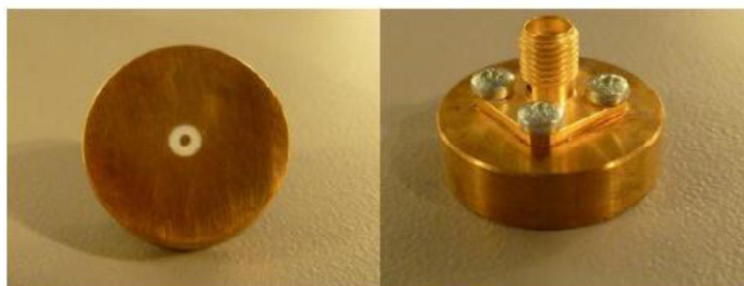
Figure 1 – MVG LIMESAR Dielectric Probe
