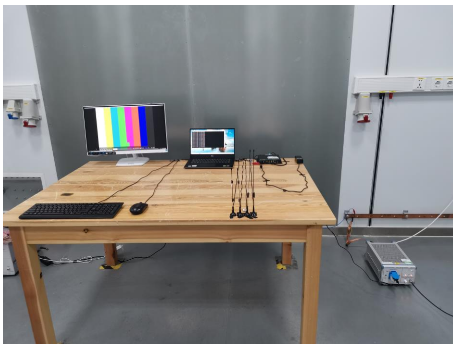
Fig. 4 Power line conducted emission setup photo
