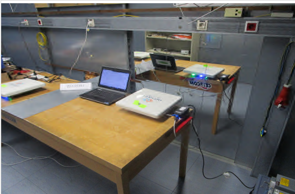
Photograph 5: EUT Test Setup, AC-Power Lines Conducted Emissions measurement
