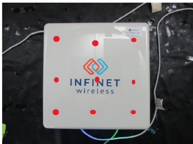
Photograph 10: Immunity test, test setup for ESD; red points: air discharge.
