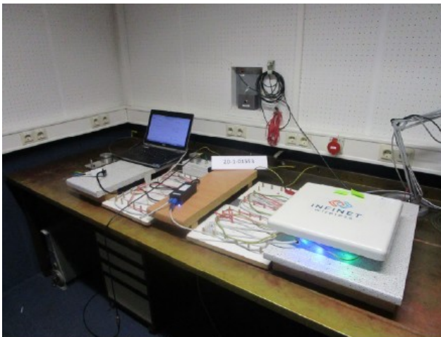
Photograph 5: conducted immunity test set-up
