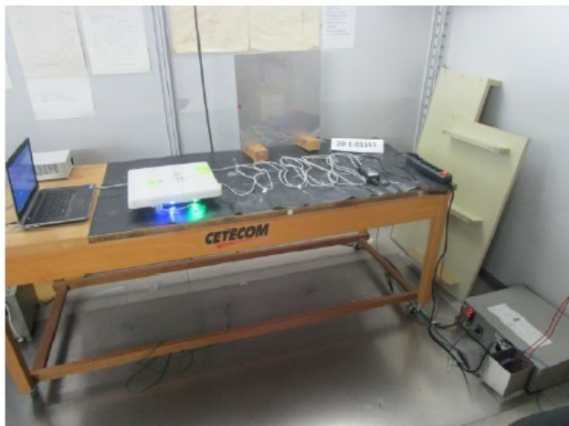
Photograph 9: Immunity test, test setup for ESD
