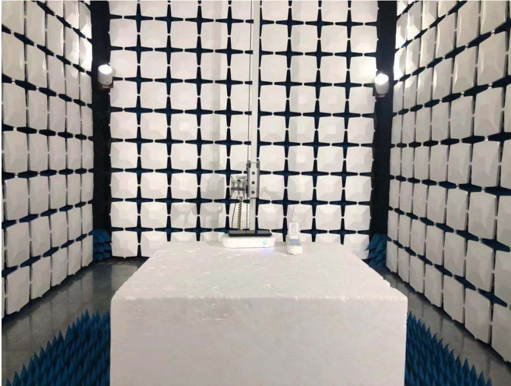
Above 1GHz for radiated emission test setup
