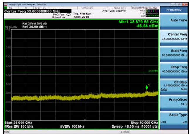
U-NII-3 ,Plot 1,Band Edge-802.11a(20M Hz),5785MHz,Ant0
