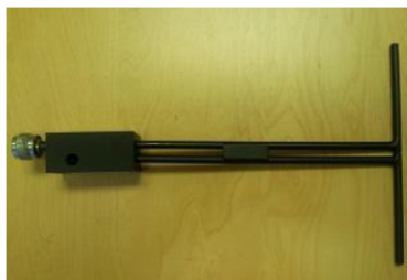
Figure 1 – MVG COMOSAR Validation Dipole
