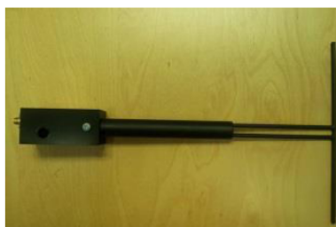
Figure 1 – MVG COMOSAR Validation Dipole
