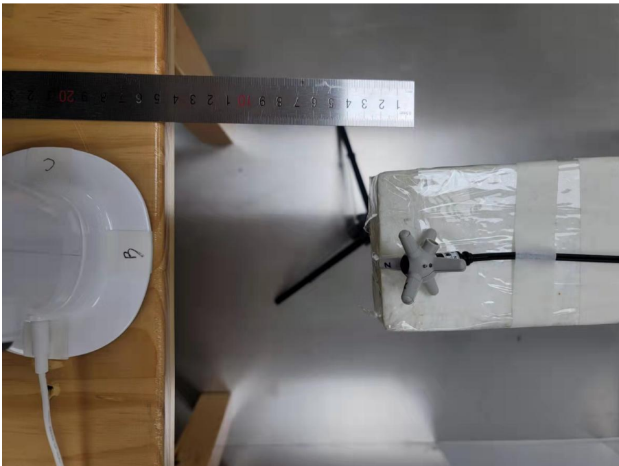
E-field Test Setup Photo of Position B(15cm)
