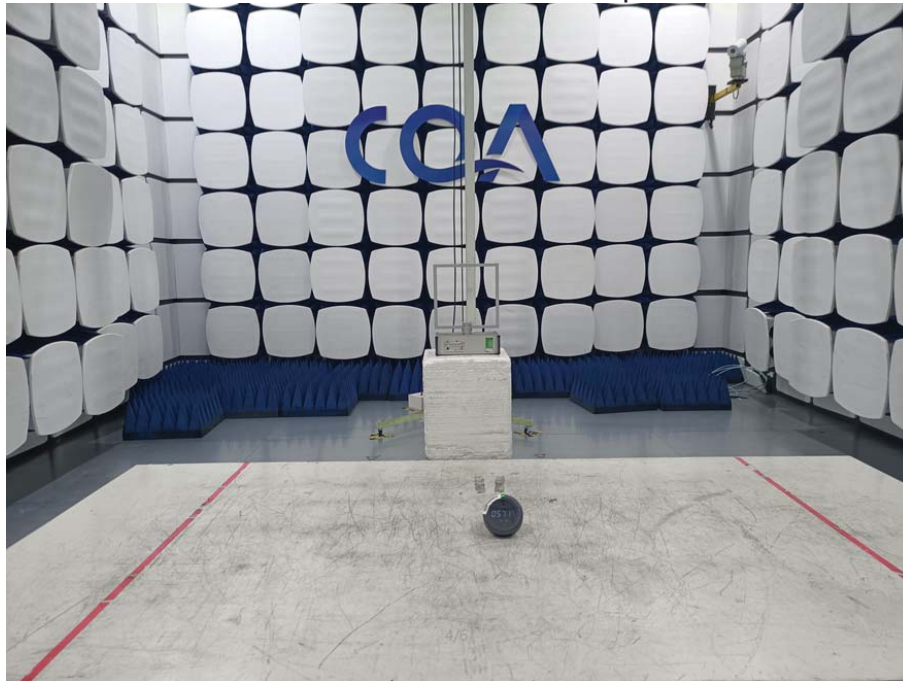
Below 30MHz Test Setup
