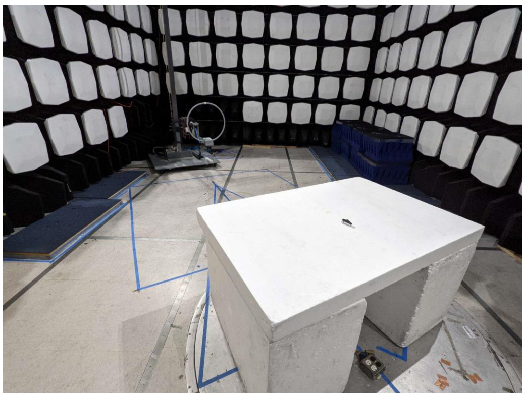
Figure 2: Equipment Under Test – Radiated Emissions <30MHz
