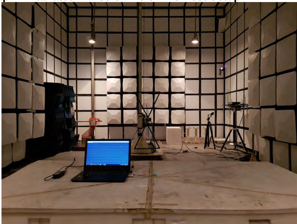
Photograph – Radiated Emission Below 1G Test Setup
