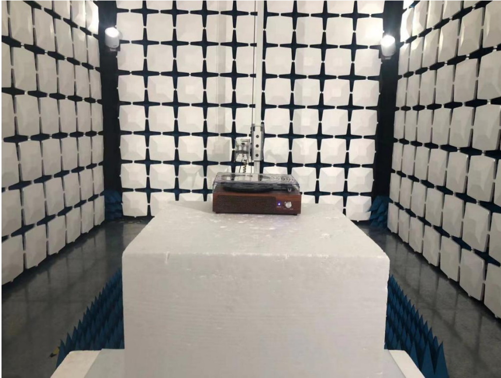
Above 1GHz for radiated emission test setup
