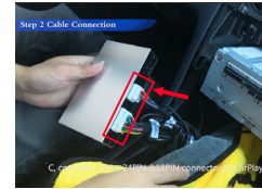
12. Connect the power cable (white one) to the carplay box, Connect the antenna cable
