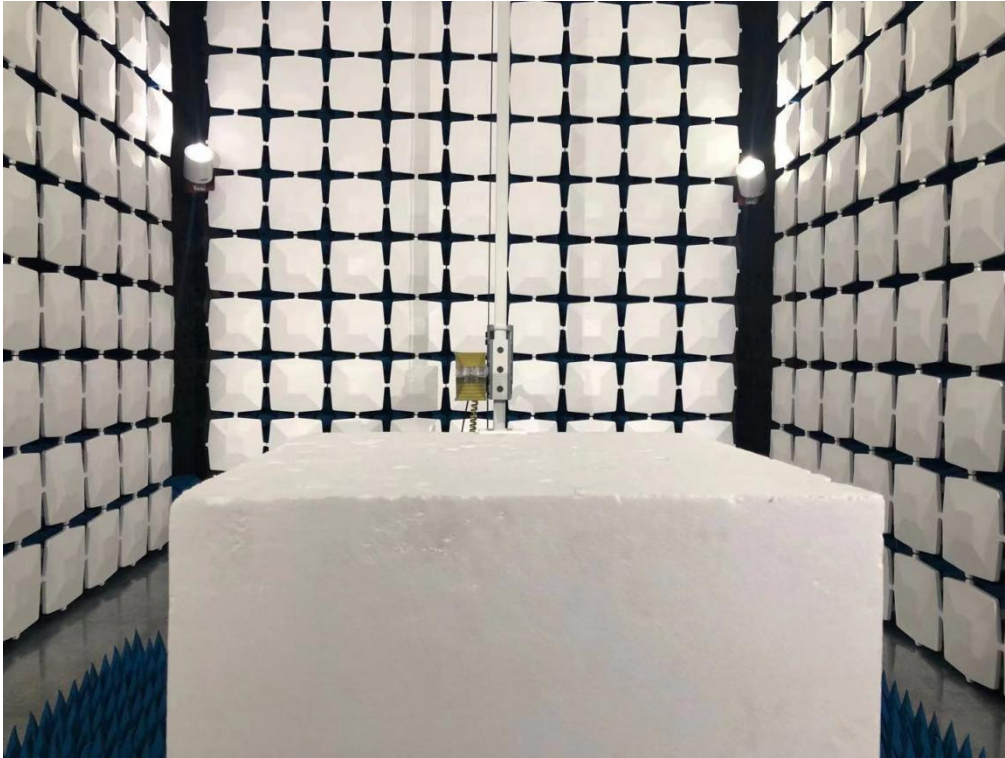
Below 1GHz for radiated emission test setup
