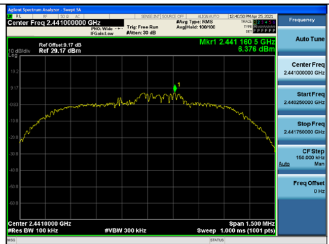
\pi/4 -DQPSK on Channel 39
