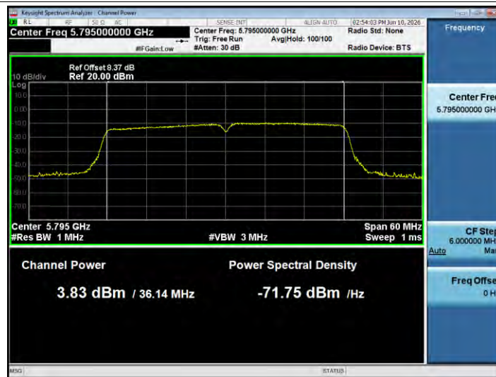
Power NVNT n40 5795MHz Ant1
