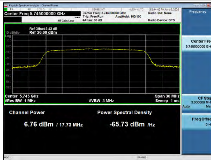
Power NVNT n20 5745MHz Ant1
