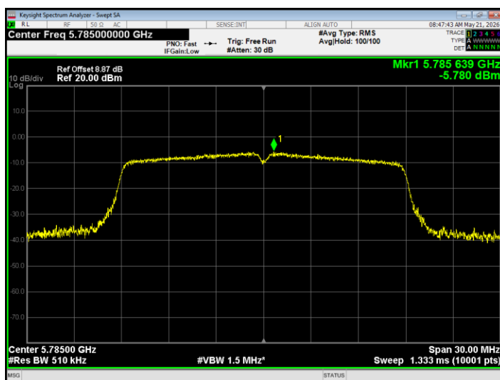
PSD NVNT n20 5785MHz Ant1
