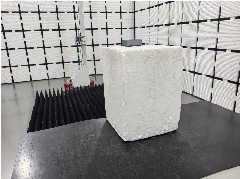
Spurious Radiation Emissions Test (>1G)
