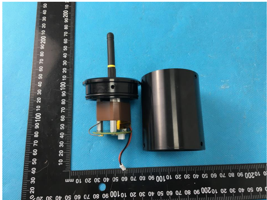
EUT Housing and Board View 3
