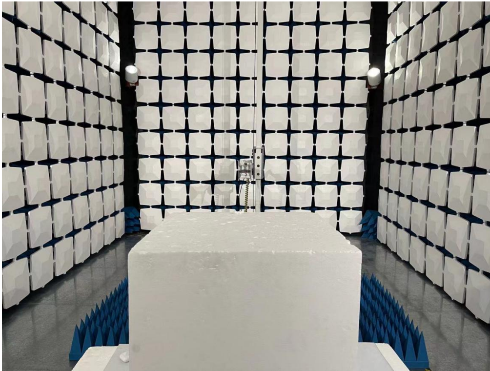
Above 1GHz for radiated emission test setup
