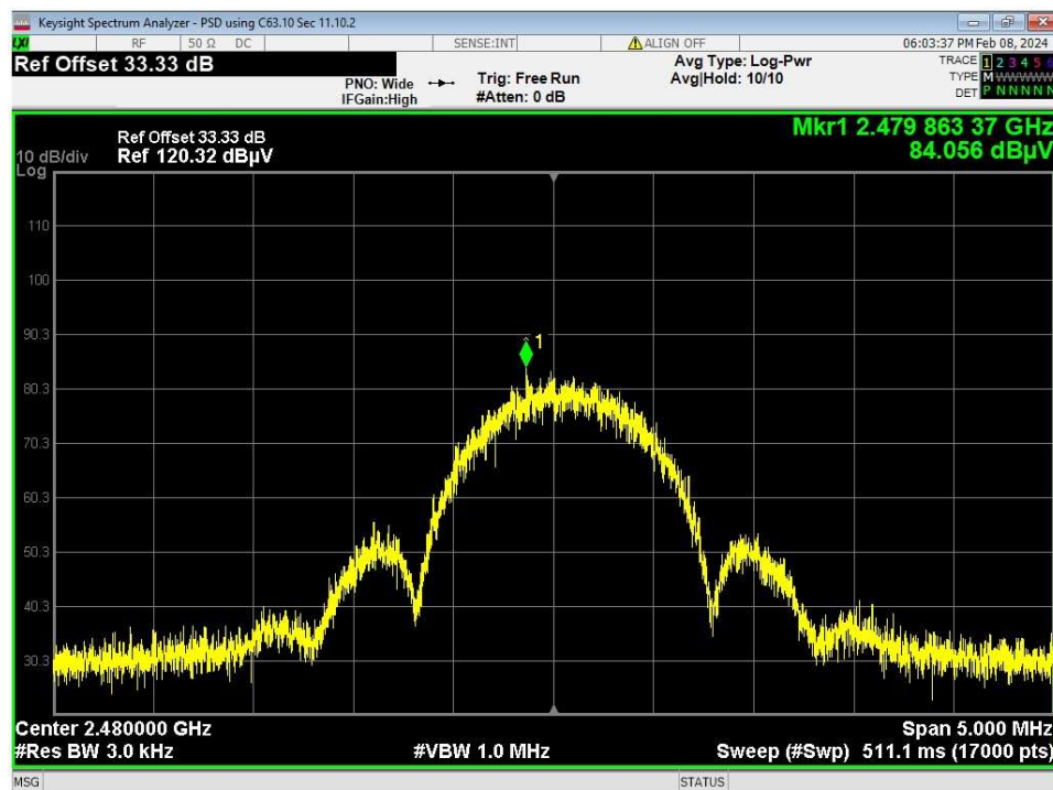
Figure 23 – EIRP Power Spectral Density, High Channel Corrected values measured at 3m.
