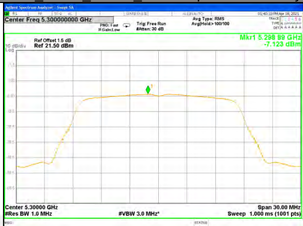
W53_11n20_Lower_Power Spectrum Density
