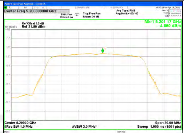
W52_11n20_Lower_Power Spectrum Density
