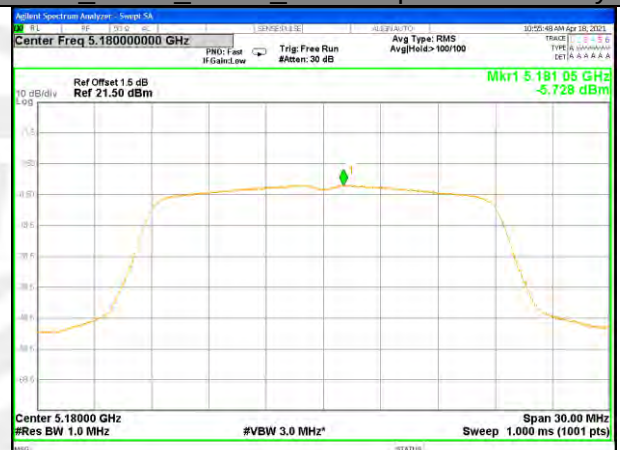
W52_11n20_Higher_Power Spectrum Density
