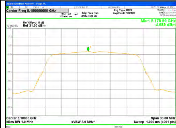
W52_11a20_Higher_Power Spectrum Density
