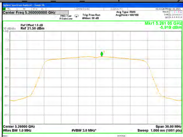
W53_11n20_Higher_Power Spectrum Density
