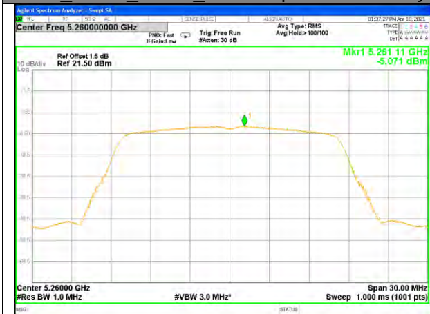
W53_11a20_Higher_Power Spectrum Density
