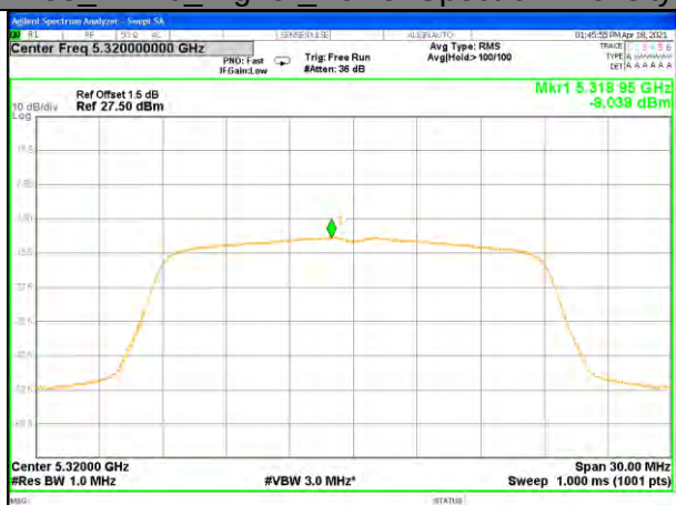
W53_11n20_Higher_Power Spectrum Density
