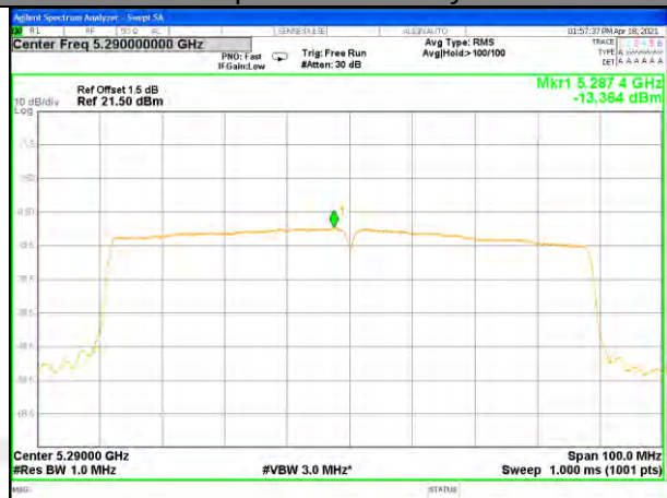
W53_11ac80_CH58(5290MHz)_Power Spectrum Density
