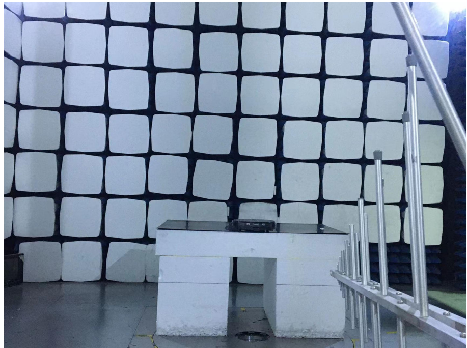
Radiation Emission Test Setup (30MHz to 1GHz)
