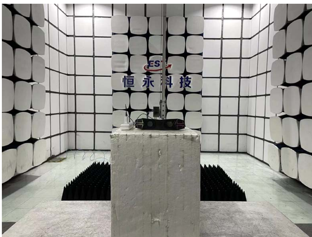
Radiated emission test: Above 1GHz
