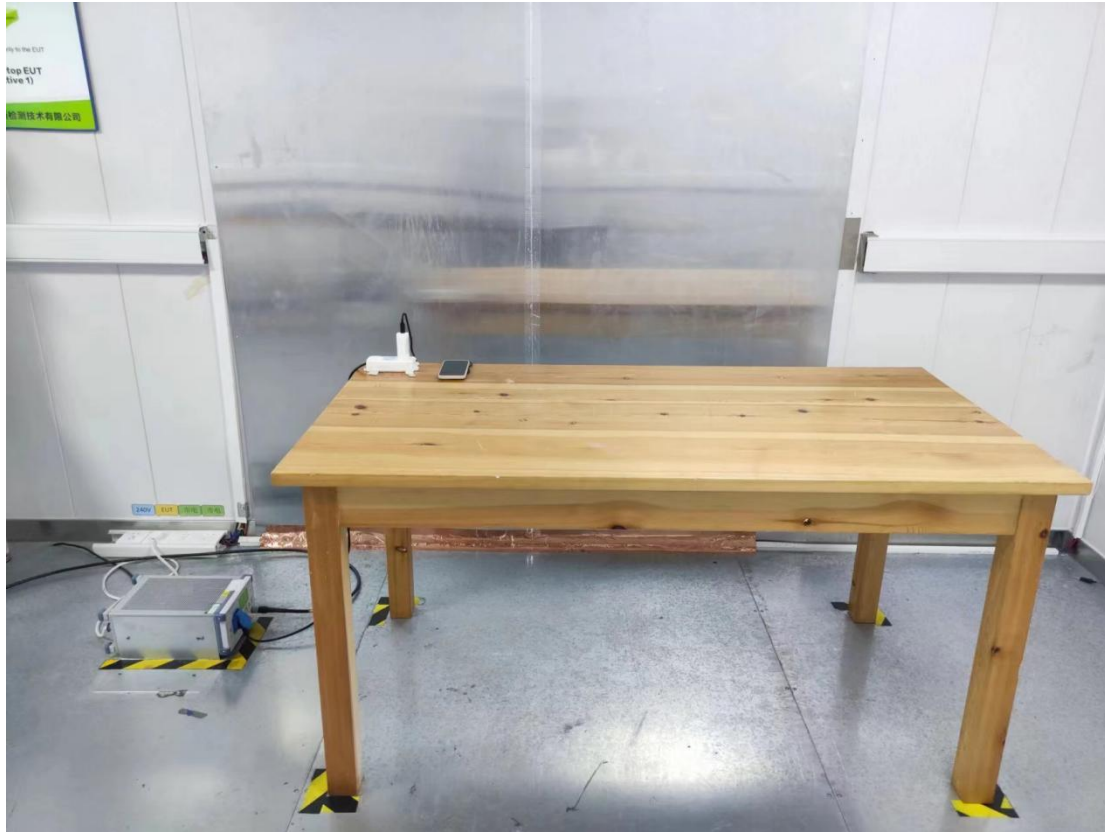
Conducted emission test setup
