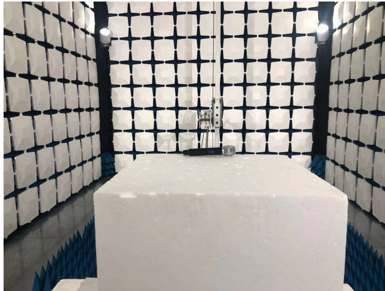
Below 1GHz for radiated emission test setup
