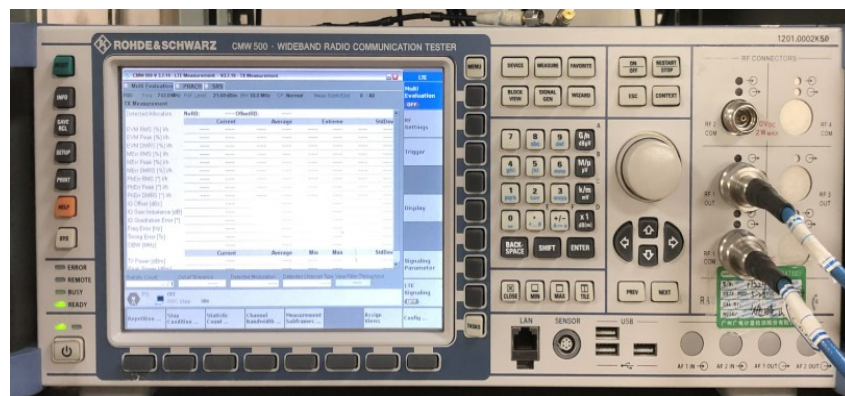
CMW 500 (2G/3G/4G Test Equipment)
