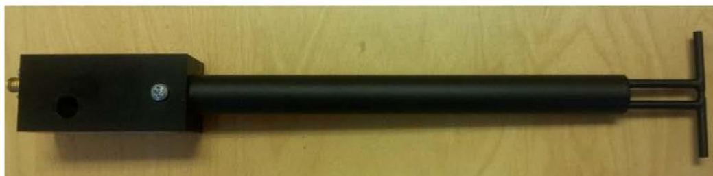
Figure 1 – MVG COMOSAR Validation Dipole
