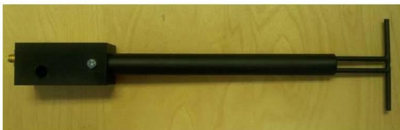
Figure 1 – MVG COMOSAR Validation Dipole
