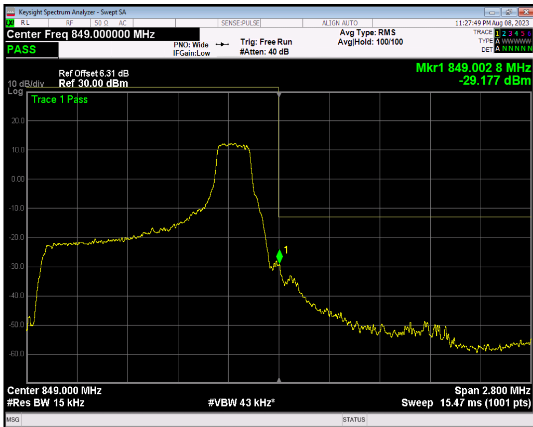
Band5 16QAM BW=1.4MHz Channel=20643 RB Size=6 Position=#0
