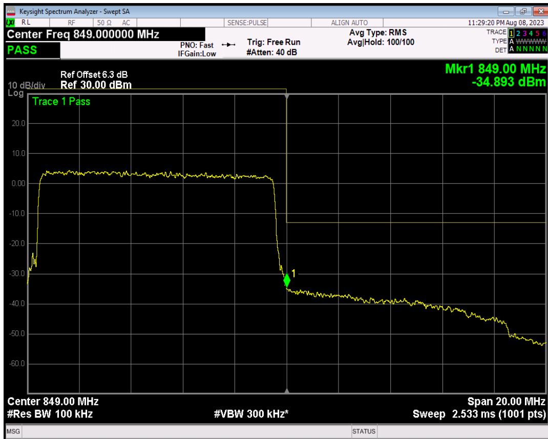
Band5 16QAM BW=10MHz Channel=20600 RB Size=1 Position=#0
