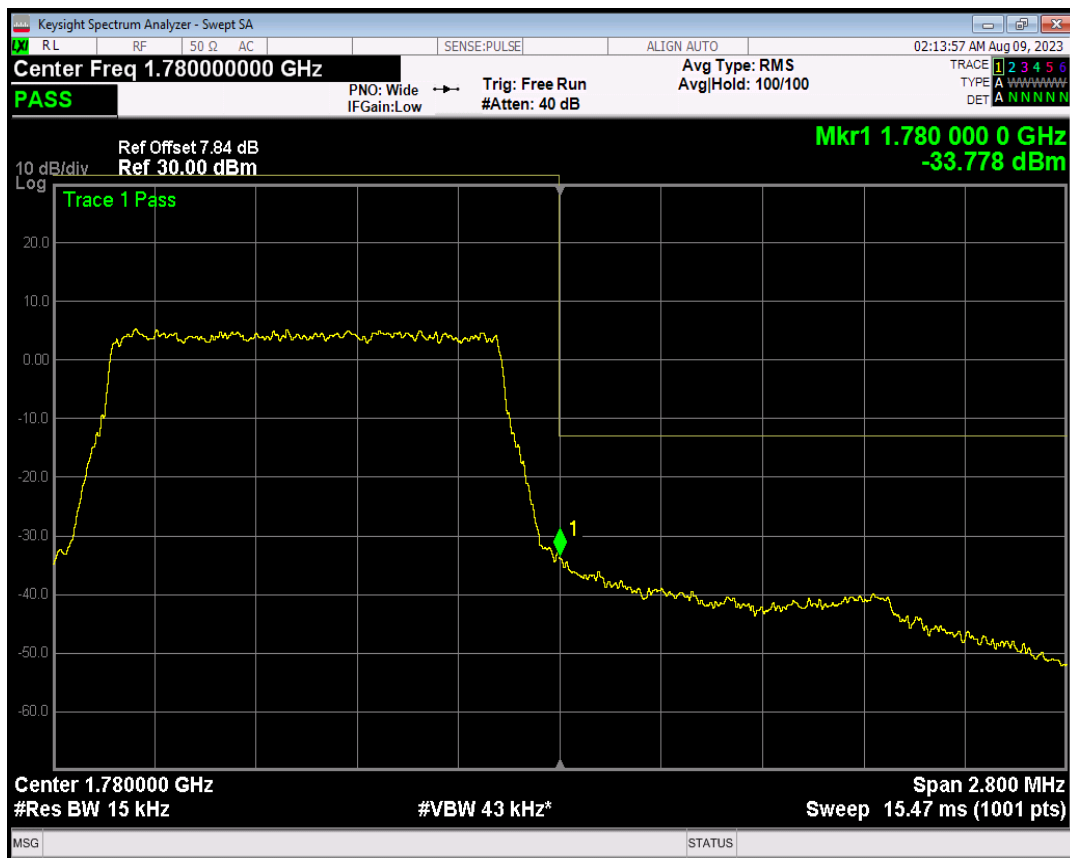
Band66 16QAM BW=1.4MHz Channel=132665 RB Size=1 Position=#0
