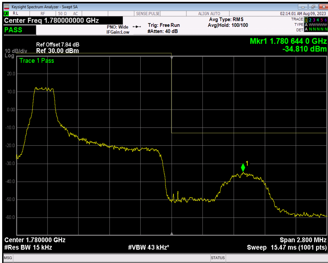
Band66 16QAM BW=1.4MHz Channel=132665 RB Size=1 Position=#Max
