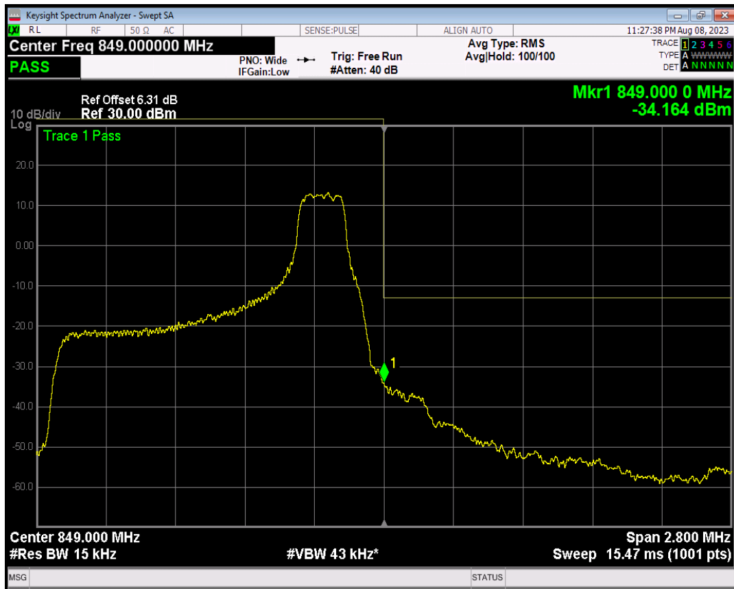
Band5 QPSK BW=1.4MHz Channel=20643 RB Size=6 Position=#0
