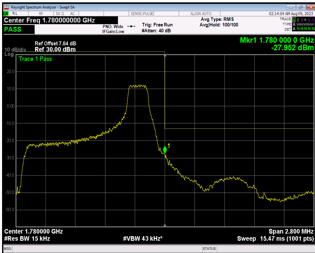
Band66 16QAM BW=1.4MHz Channel=132665 RB Size=6 Position=#0
