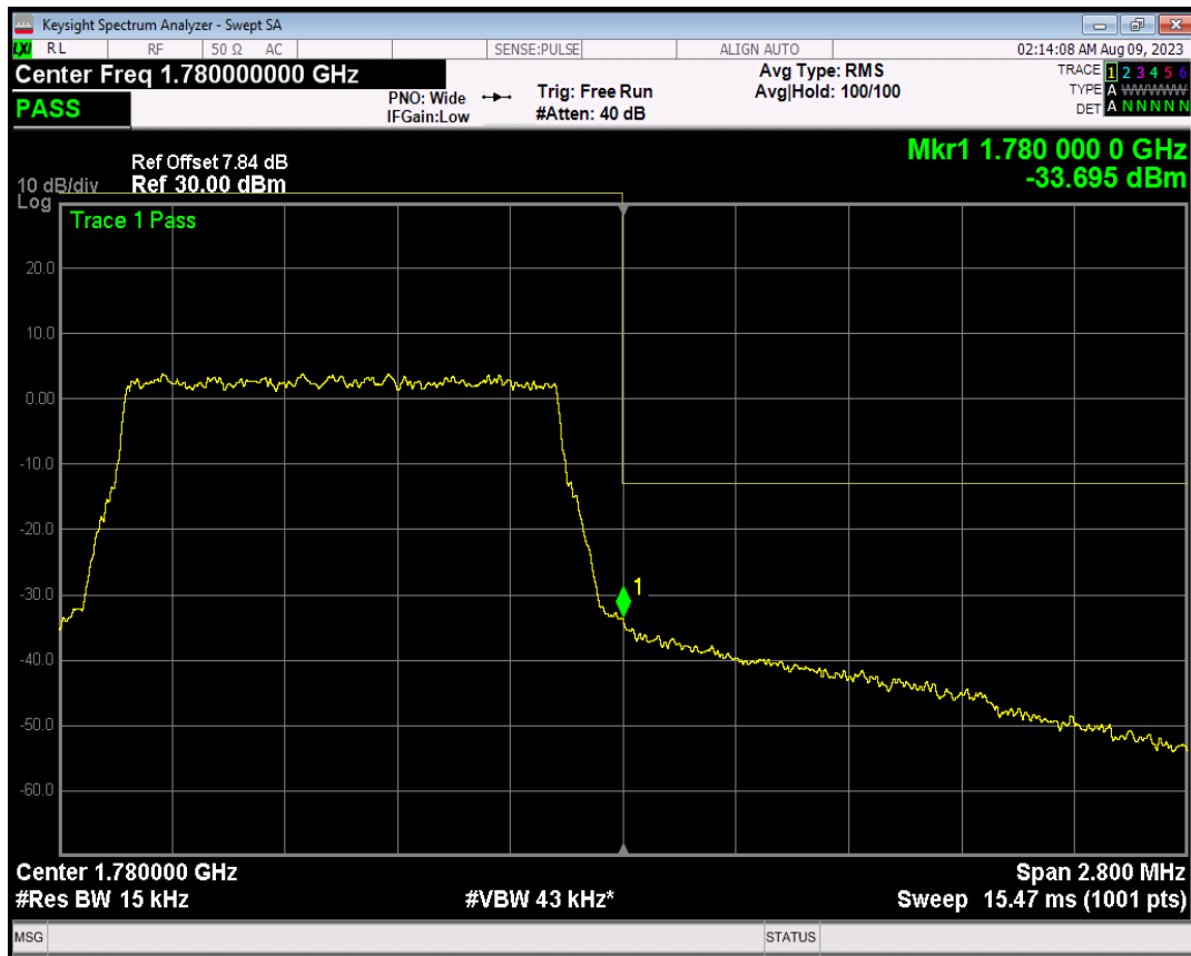
Band66 QPSK BW=3MHz Channel=131987 RB Size=1 Position=#0
