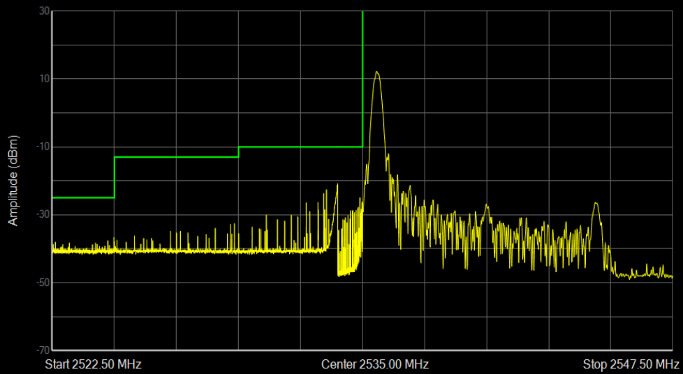
Band41(2535-2655) QPSK BW=10MHz Channel=40090 RB Size=1 Position=#0
