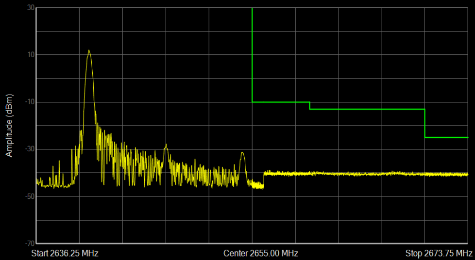
Band41(2535-2655) QPSK BW=15MHz Channel=41165 RB Size=1 Position=#0
