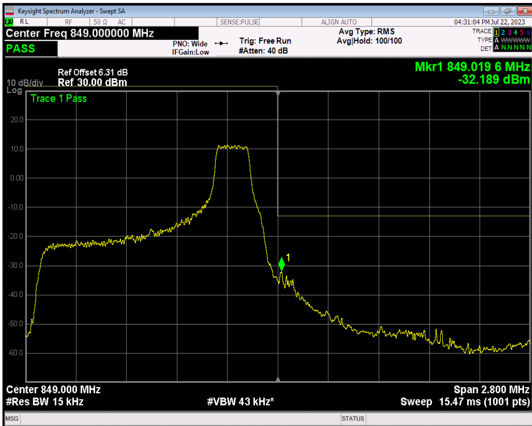
Band5 16QAM BW=1.4MHz Channel=20643 RB Size=6 Position=#0
