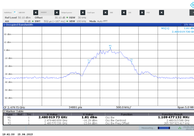
Figure 7.5-6: 99% occupied bandwidth on high channel
