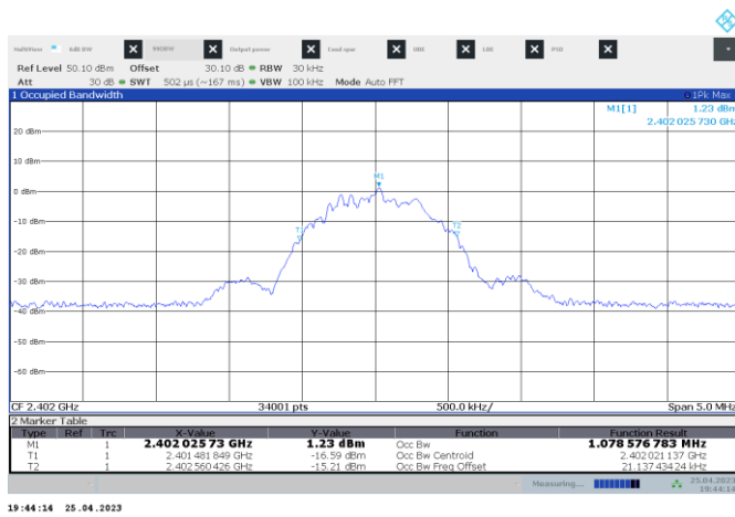
Figure 7.5-4: 99% occupied bandwidth on low channel
