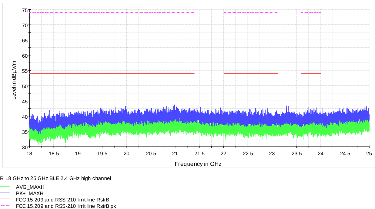
Figure 7.7-11: radiated spurious emissions from 18 GHz to 25 GHz at high channel
