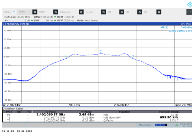
Figure 7.5-1: 6 dB bandwidth on low channel
