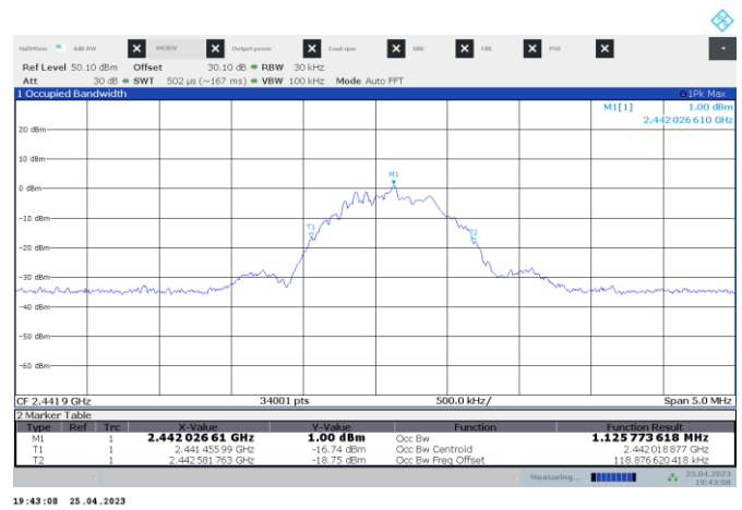
Figure 7.5-5: 99% occupied bandwidth on mid channel
