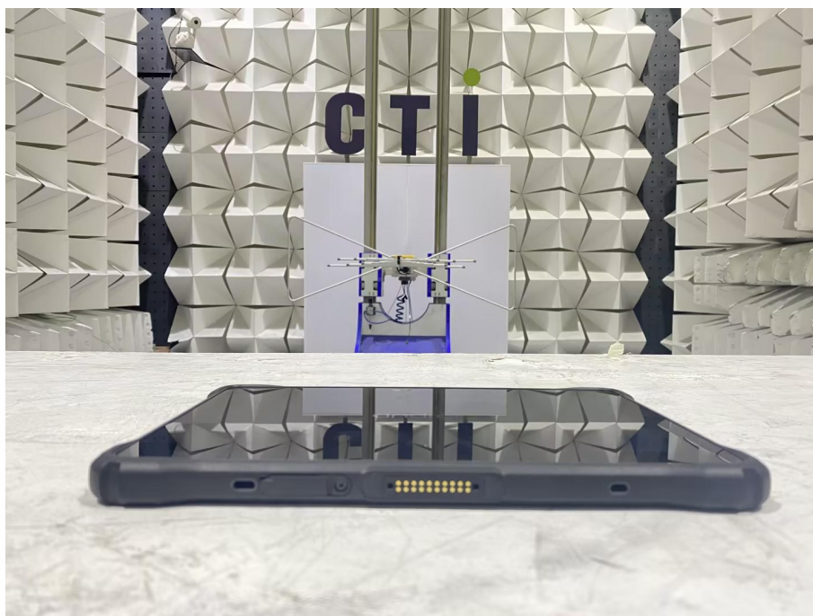
Radiated spurious emission Test Setup-2(Below 1GHz)
