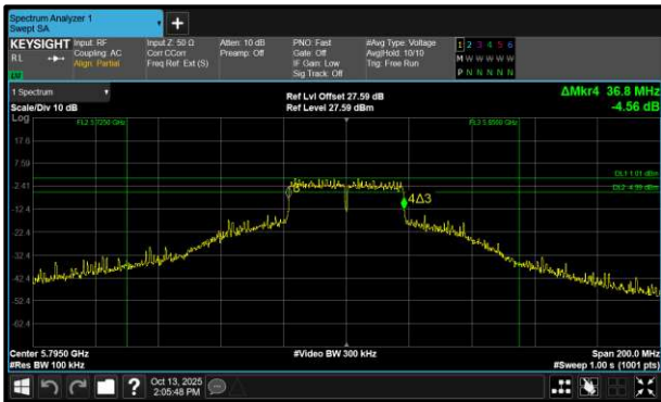
Figure 59 - B 5795 MHz (CH159) 6 dB Bandwidth
