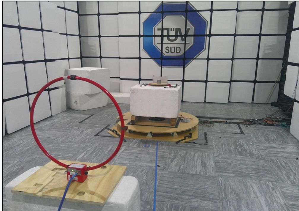
Figure 19 - Test Setup - 9 kHz to 30 MHz
