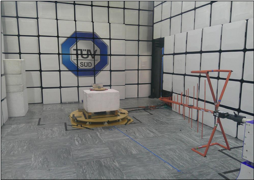
Figure 10 - Test Setup - 30 MHz to 1 GHz
