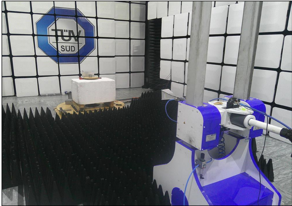
Figure 12 - Test Setup - 8 GHz to 18 GHz
