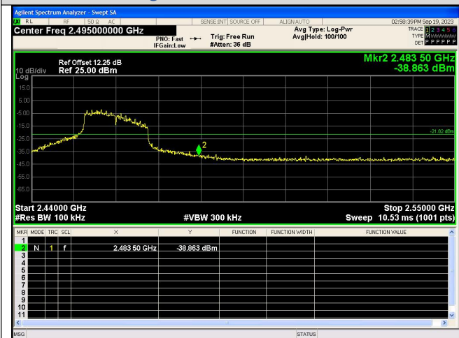
Out Of Band Emission IEEE 802.11g_Channel 11_20MHz_Antenna 0
