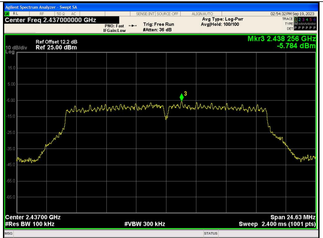
In-Band Reference Level IEEE 802.11g_Channel 6_20MHz_Antenna 0
