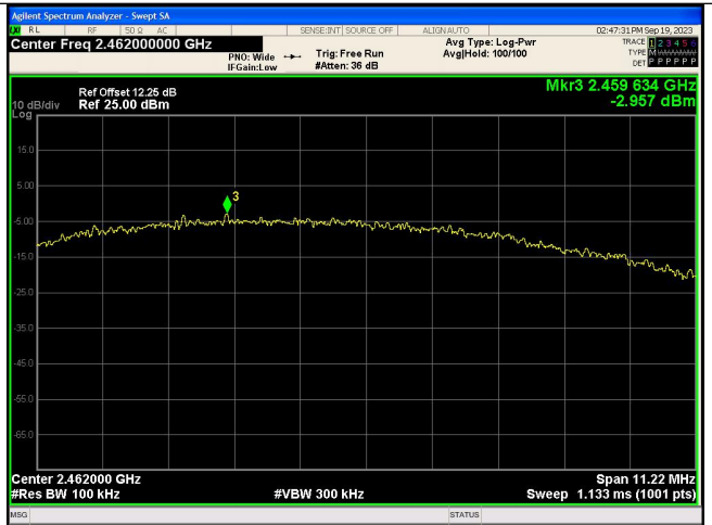
In-Band Reference Level IEEE 802.11b_Channel 11_20MHz_Antenna 0
