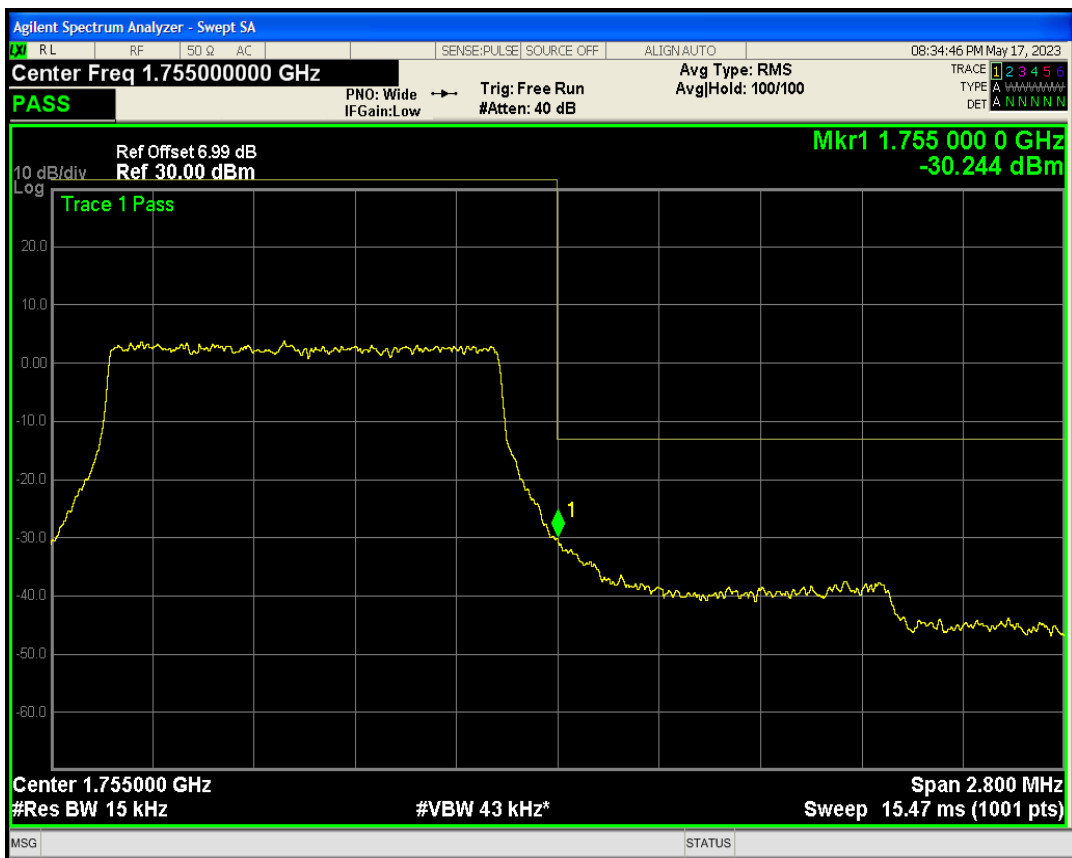
Band4 QAM16 BW=1.4MHz Channel=20393 RB Size=6 Position=#0
