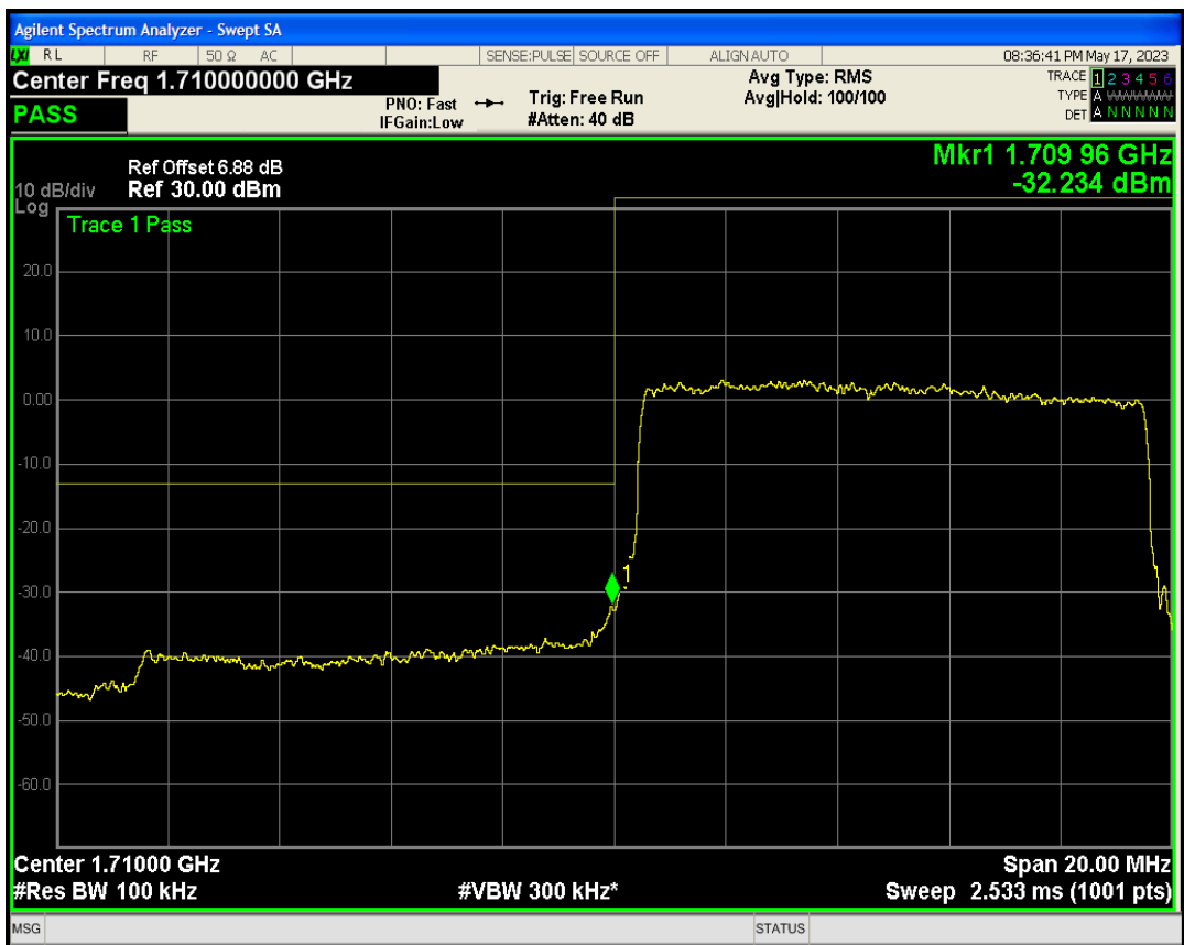
Band4 QAM16 BW=10MHz Channel=20000 RB Size=50 Position=#0
