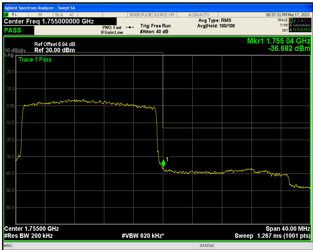
Band4 QAM16 BW=20MHz Channel=20300 RB Size=100 Position=#0
