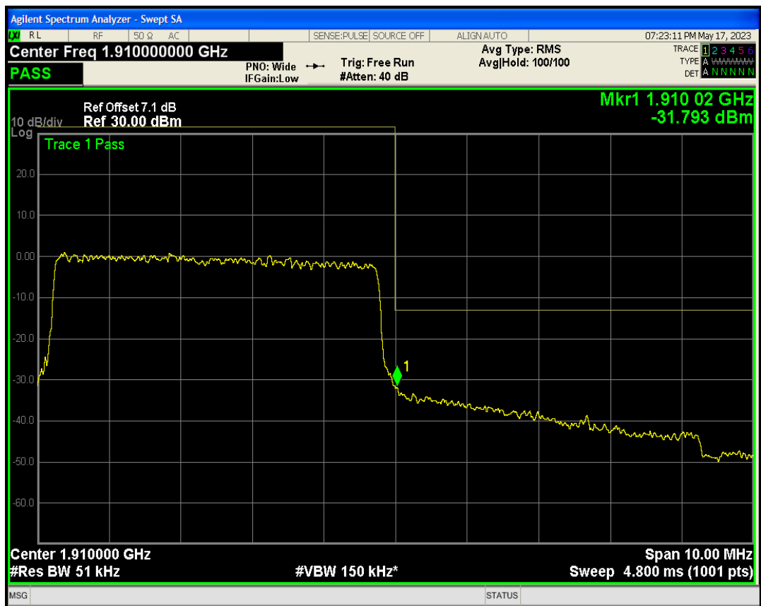
Band2 QAM16 BW=5MHz Channel=19175 RB Size=25 Position=#0
