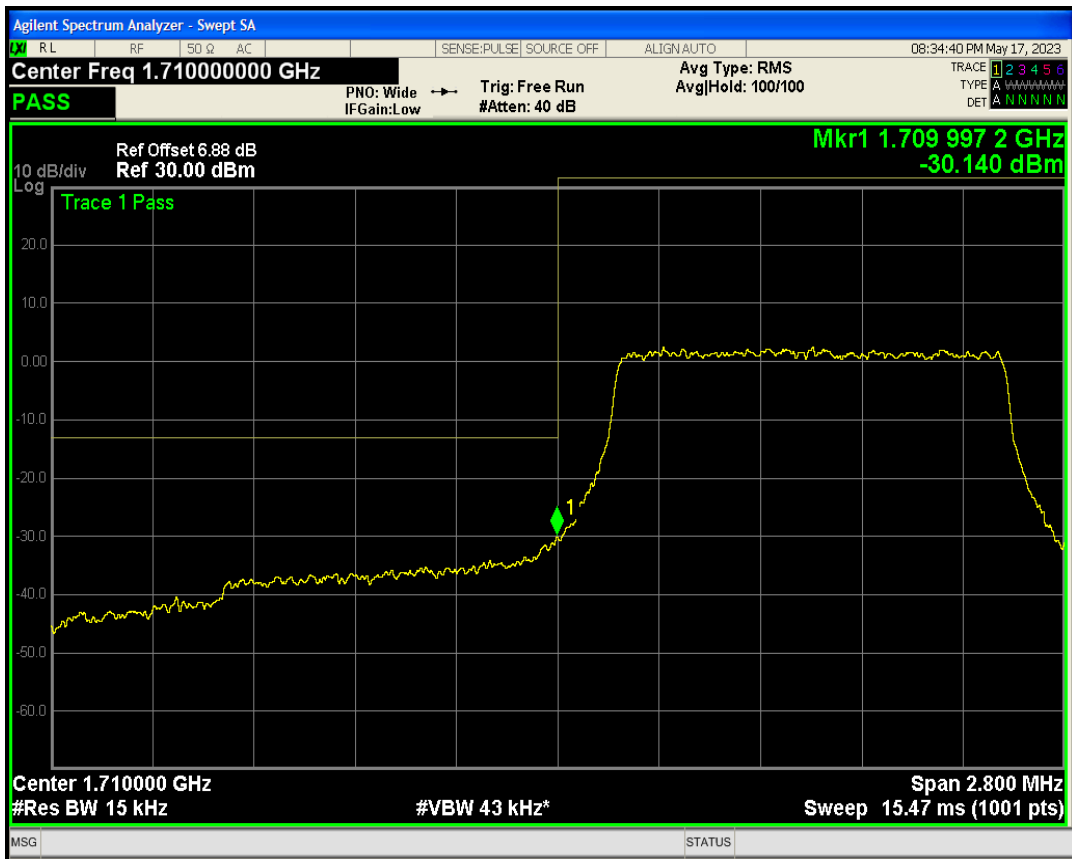
Band4 QPSK BW=1.4MHz Channel=20393 RB Size=6 Position=#0
