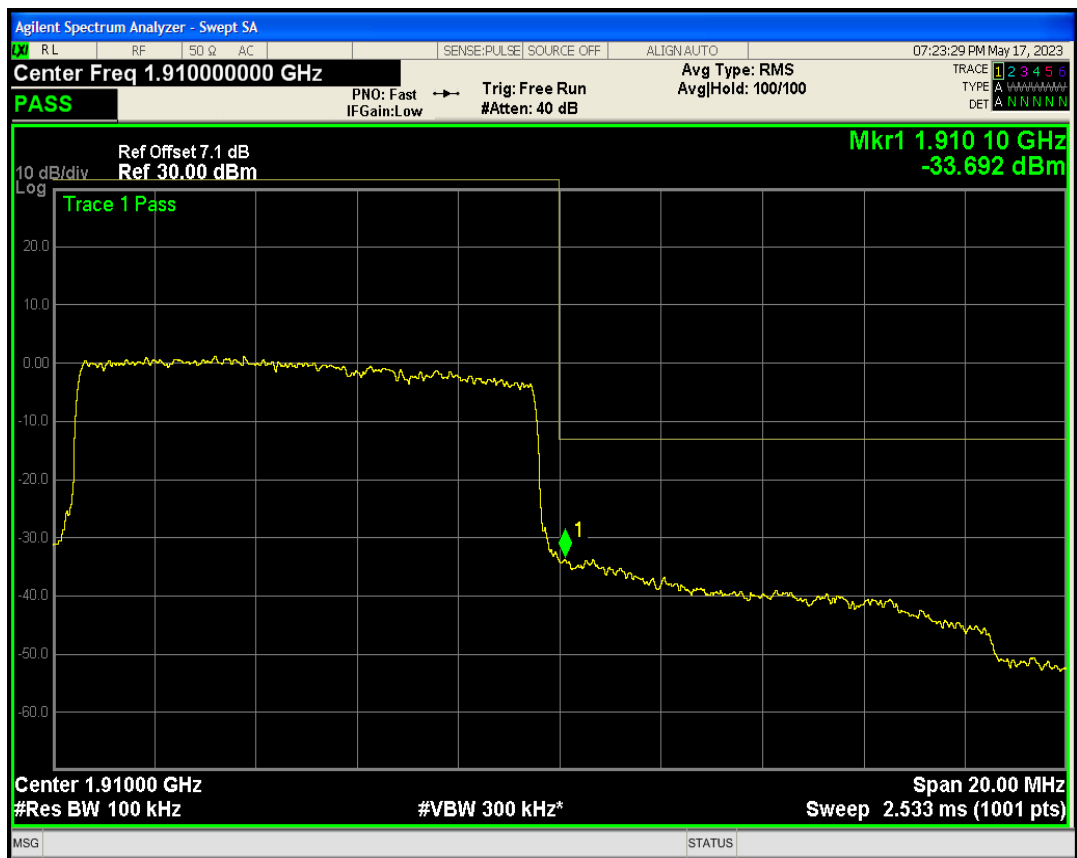
Band2 QAM16 BW=10MHz Channel=19150 RB Size=50 Position=#0
