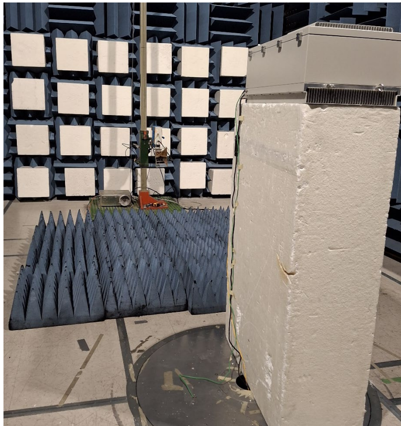
Figure 4: Radiated Emissions (Above 1GHz) Emissions Test Setup
