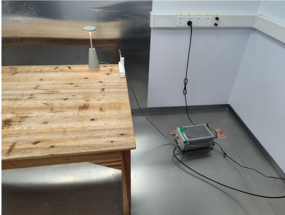
Photo of Conducted Emission Measurement
