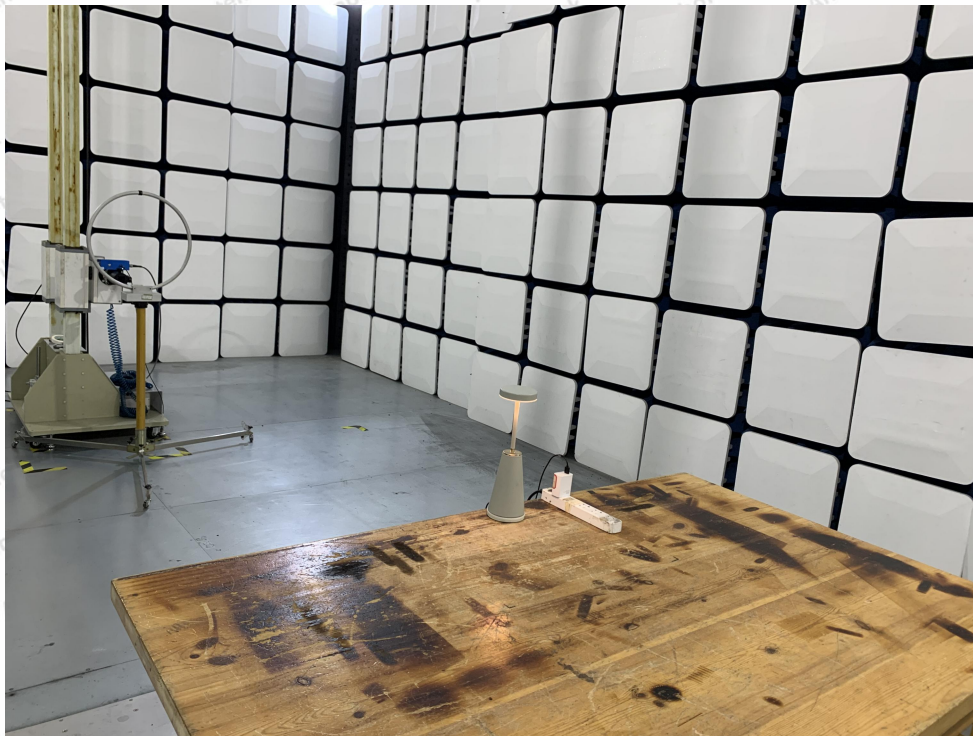
Photo of Radiation Emission Test
