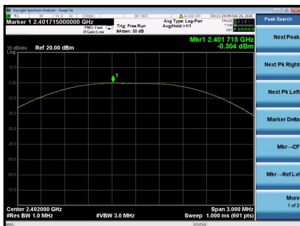
GFSK (BLE 1Mbps) LOW CHANNEL
