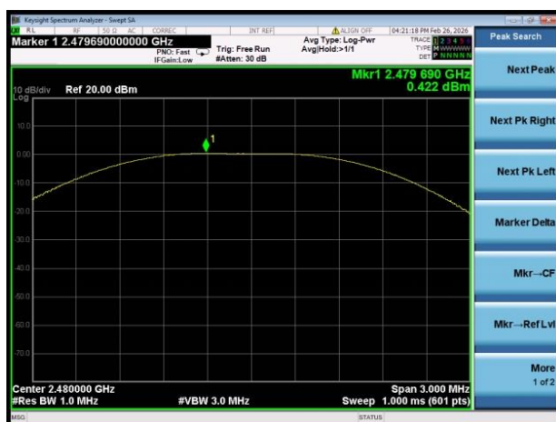
GFSK (BLE 1Mbps) HIGH CHANNEL
