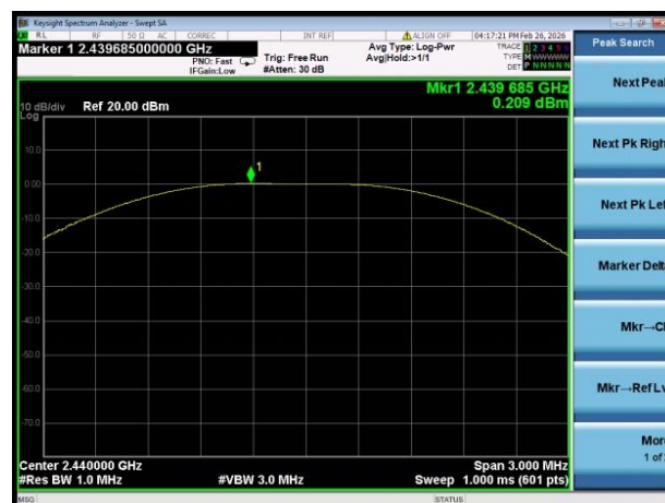
GFSK (BLE 1Mbps) MIDDLE CHANNEL
