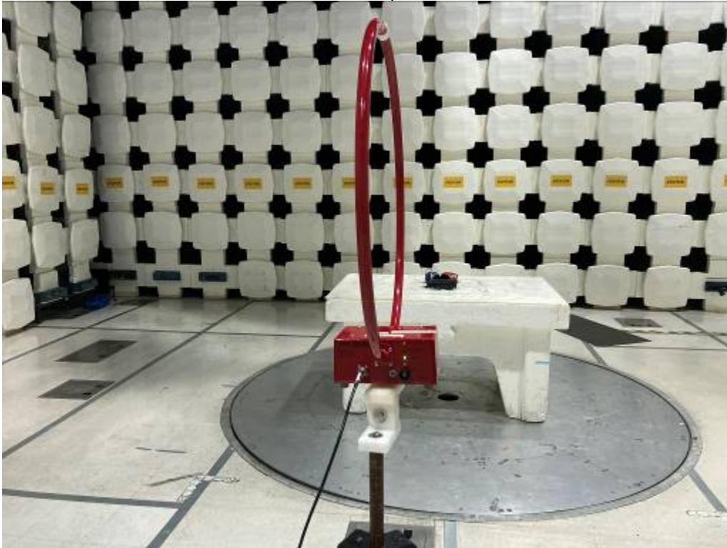
Radiated Emissions Test Setup, 9 kHz-30 MHz, Z-Axis
