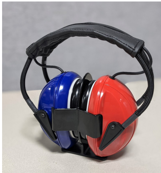
Figure 4.1: WAHTS on Calibration Check Fixture . To place the WAHTS in the calibration fixture, hold the WAHTS above the fixture with the ear cushions almost touching. Gently slide the WAHTS vertically down into the fixutre.
