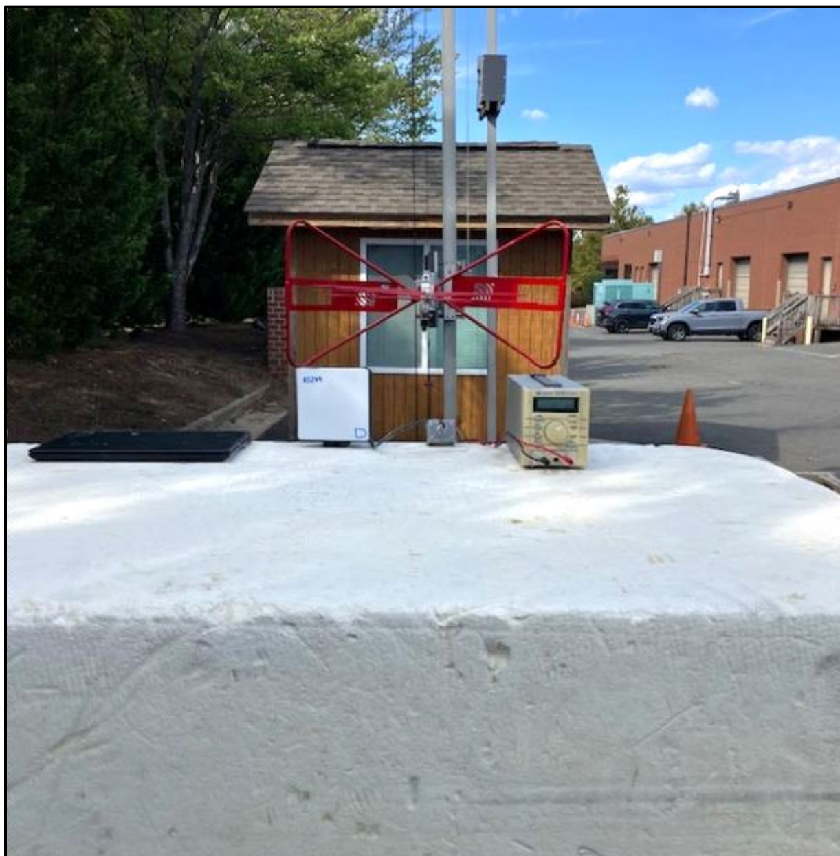
Photograph 5: Radiated Emissions Test Setup >1 GHz, Front View
