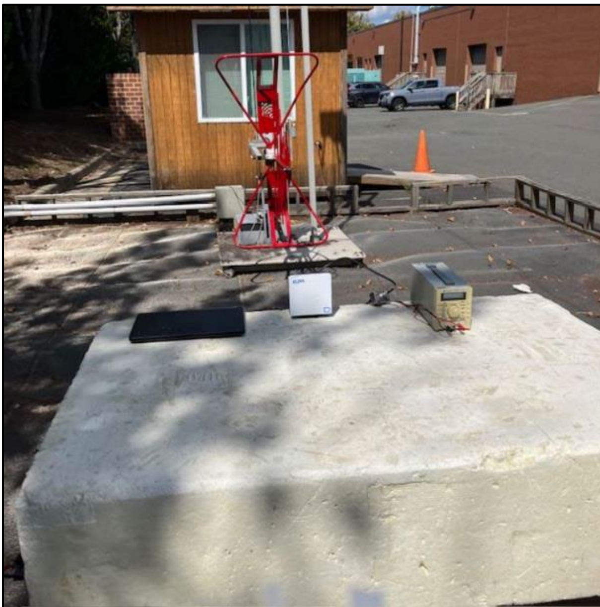
Photograph 3: Radiated Emissions Test Setup <1 GHz, Front View
