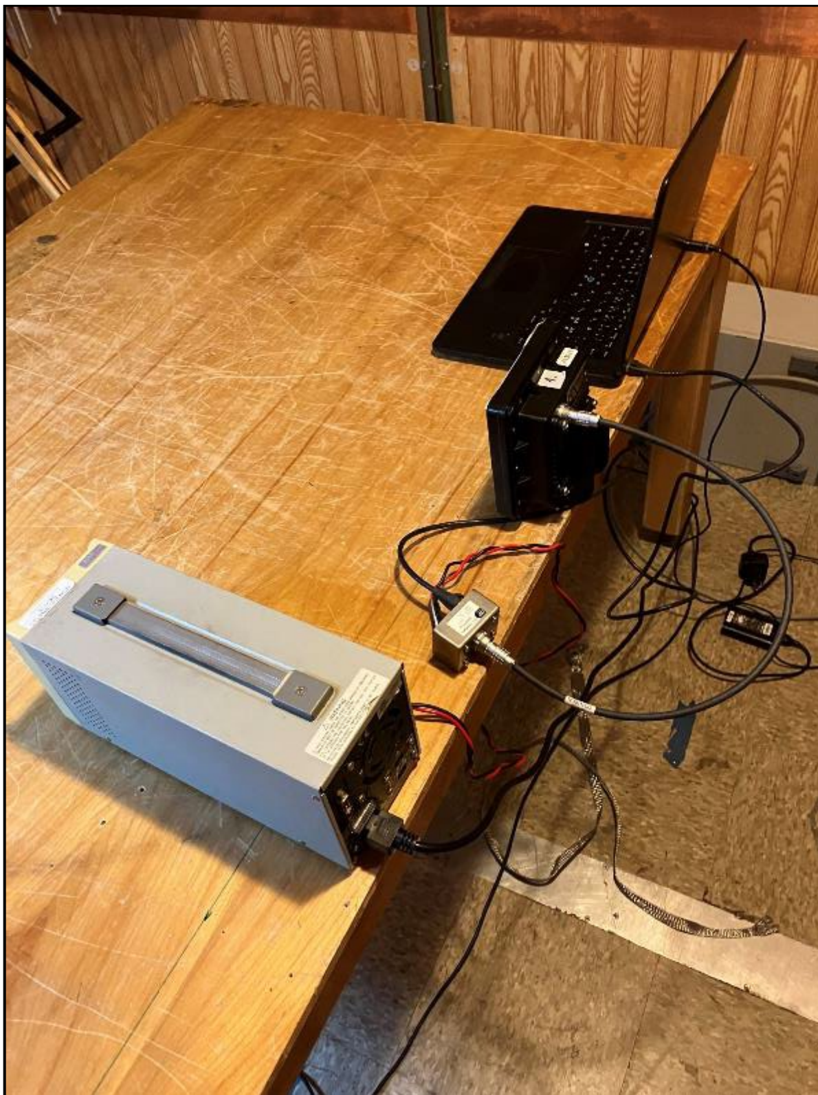
Photograph 2: Conducted Emissions Test Setup, Rear View
