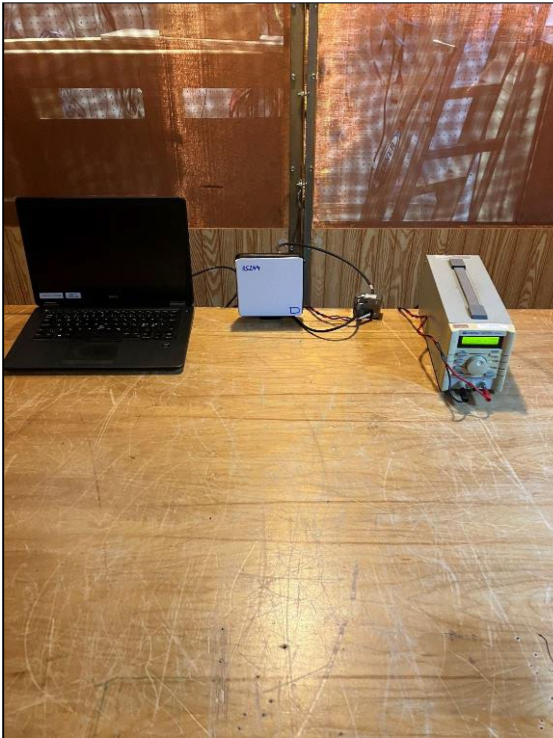
Photograph 1: Conducted Emissions Test Setup, Front View
